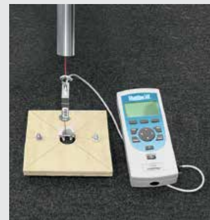
Testing of fixing element strength
