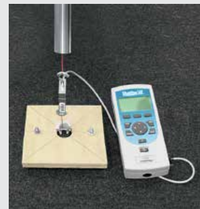
Testing of fixing element strength
