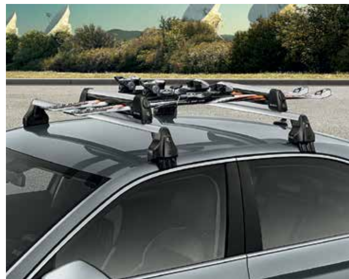
Lockable ski or snowboard rack with aluminium profile (000 071 129H)
