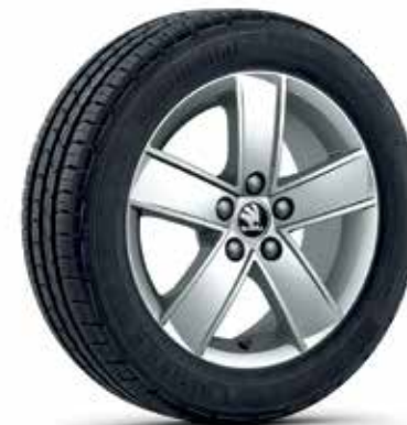
Propeller 5JA 071 495A 8Z8 light-alloy wheel 6.0J × 15" ET38 for 185/60 R15 tyres, silver metallic ŠKODA Genuine Accessories
