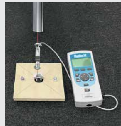
Testing of fixing element strength
