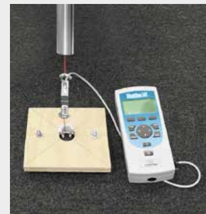
Testing of fixing element strength
