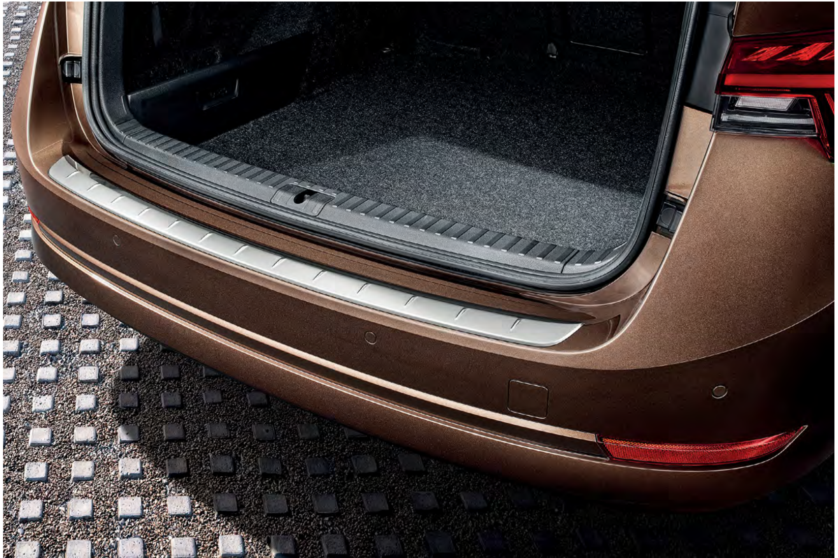
Loading edge protection strip – stainless steel
